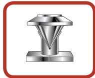
Flares rolled out above die bar.
